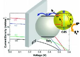
performance. QDSC constructed with Mn-doped-CdS/CdSe deposited on mesoscopic  $TiO_2$  film as photoanode,  $Cu_2S$ /Graphene Oxide composite electrode, and sulfide/polysulfide electrolyte deliver power conversion efficiency of 5.4%.
