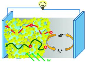
charge separation. Disparity between the electron and hole scavenging rate leads to further accumulation of holes within the CdSe QD and increases the rate of electron-hole recombination. To overcome the losses due to charge recombination processes at the interface, researchers need to accelerate electron and hole transport.
